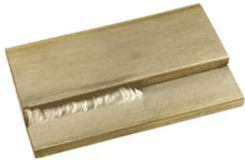
A Lap weld made on the course
