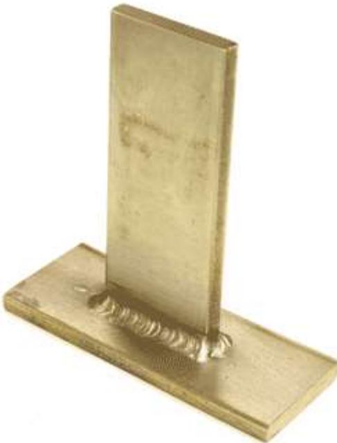
A Fillet weld made on the course
