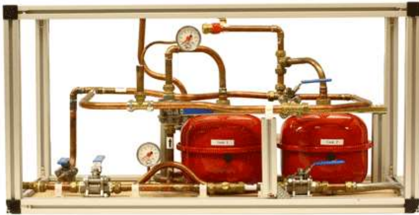
One of the practical rigs used on the Line Breaking course, helping candidates gain meaningful practice of line breaking pipework isolation procedures
