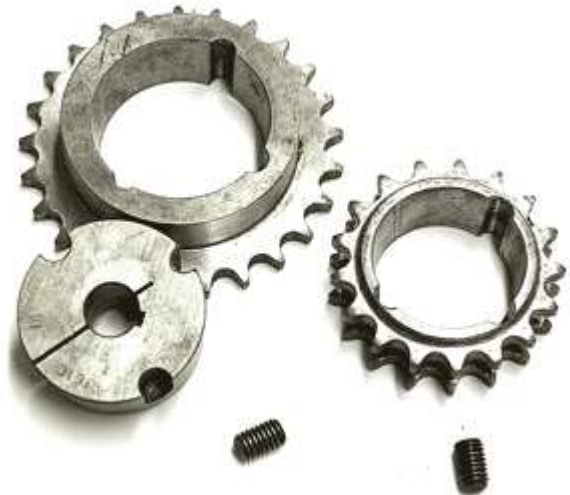
A range of sprocket drives, taper-lock bushes and pulleys are used to teach candidates how to detect for wear, how to ensure correct fitting, etc
