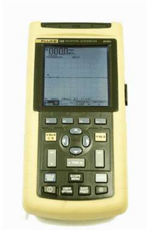
The digital storage oscilloscope used on the inverter drives training course
