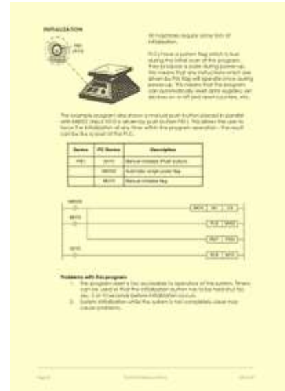
Page 14 of the course notes for the PLC Programming course, which is part of a section where we discuss various PLC applications and how a PLC would be programmed to control them. This particular example is explaining how system flags are often used to initialize programs, by setting counters and other registers to a default state when the program is initiated
