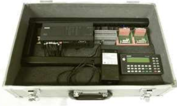
The Siemens S7 PLC used on the PLC training courses
