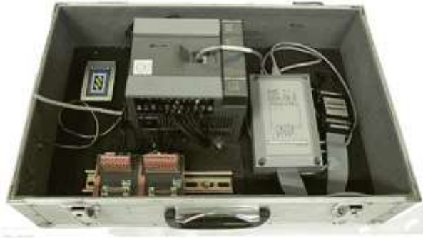
The Allen Bradley SLC500 PLC used on the PLC training courses
