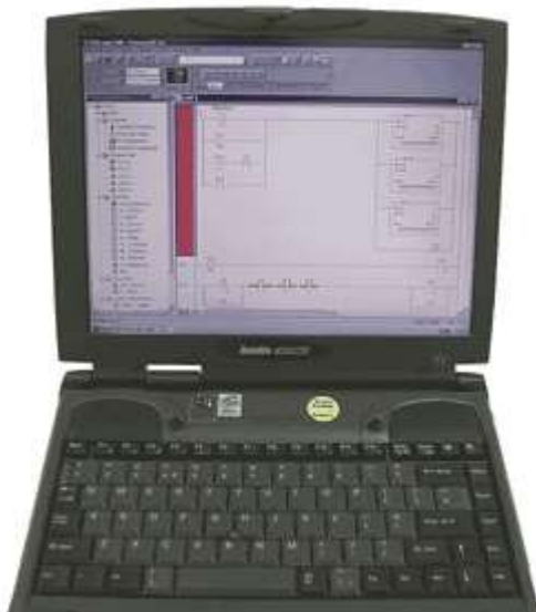
The Allen Bradley RS Logix PC-based software package used on the PLC training courses
