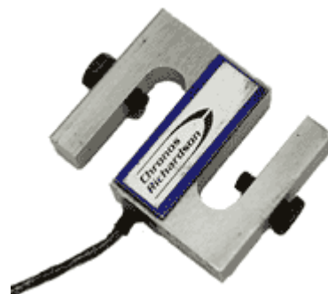
One of the 4-wire load cells used on the instrumentation training course
