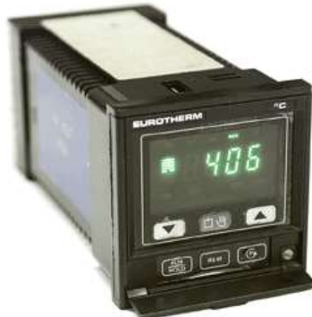
One of the Eurotherm controllers used on the control and instrumentation training course
