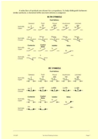
Page 17 of part 2 of the course notes for the electrical maintenance training course, describing the various electrical symbols used on drawings for a range of common Standards
