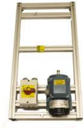
This is one of the specially-wound 40 volt three-phase motors used on the electrical maintenance training course
