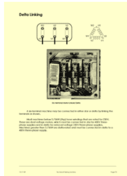
Page 13 of part 2 of the electrical maintenance training course notes, describing the configuration of the terminals of a delta-linked motor
