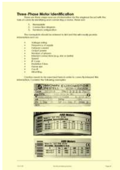
Page 9 of part 2 of the electrical maintenance training course notes, describing the information found on the nameplates of industrial motors
